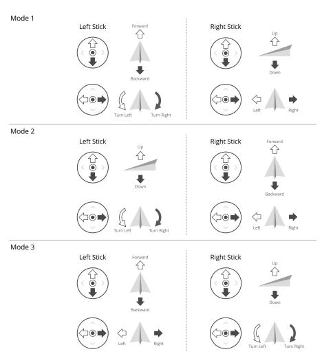
The default control mode of the remote controller is Mode 2. In this manual, Mode 2 is used as an example to illustrate how to use the control sticks.
