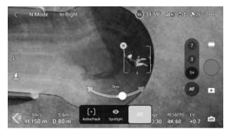
c. Tap on the bottom of the screen to switch to ActiveTrack. In Trace mode, the tracking direction can be changed using the direction wheel (Front, Back, Left, Right, Front Diagonal Left, Front Diagonal Right, Back Diagonal Left, and Back Diagonal Right). The direction wheel will be minimized if there is no operation for an extended period or any other area of the screen is tapped.
