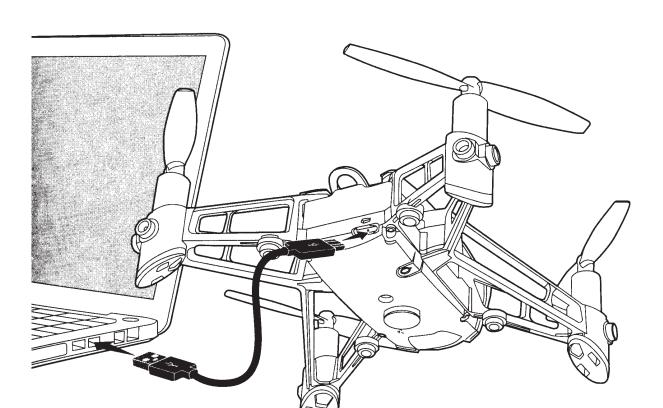
The charge LED is steady red when charging.
